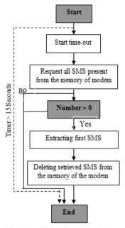
Figure 10. Flow Chart for Receiving Routine.
