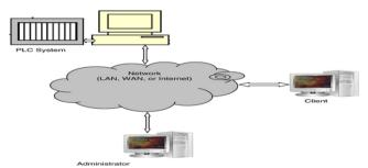
Figure 1. PC-based remote accessibility
