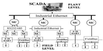
Figure 2. Network deployment in an industrial plant
