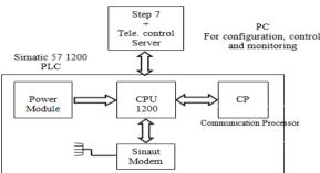
Figure 7. System Architecture for the Prototype Model.
